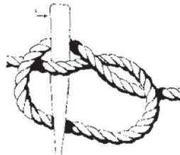
Marlin spike hitch - should not be used for sending tools or materials aloft. A tools is to open up the rope and push tool through.
