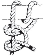
Round turn and two half hitches - widely used for securing running ends of tackles. The more turns made before hitches are made the more control is possible.
