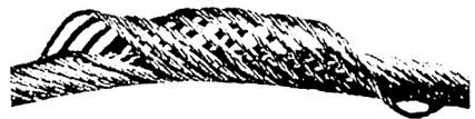
8. Typical example of localised wear and deformation created at a previously kinked portion of rope.
