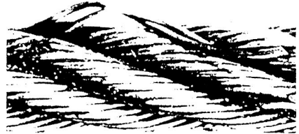
7. Wire fractures at the strand, or core interface, as distinct from 'crown' fractures, caused by failure of core support.
